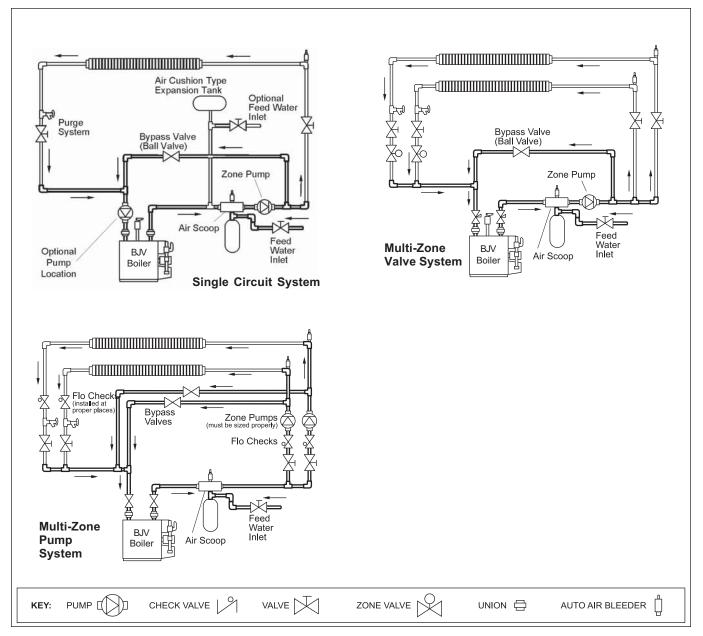
Figure 6A. Typical Plumbing Installations.
